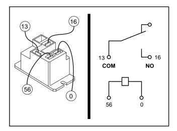
Figure 7. The Starter Contactor Relay
